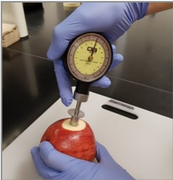
Figure 2. An Effegi firmness tester/penetrometer with a 7/16-inch diameter plunger used to measure firmness in one side of an apple. Photo: Macarena Farcuh, University of Maryland.
