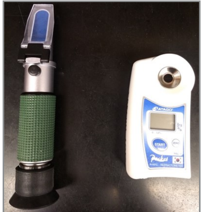
Figure 6. A hand-held manual refractometer (left) and digital refractometer (right) measure soluble solids contents of an extracted fruit apple juice sample. Photo: Macarena Faruh, University of Maryland.
