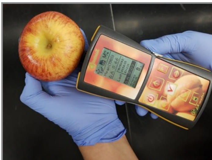
Figure 1. Using a DA meter to quantify the Index of Absorbance Difference ( I_{AD} ) which relates to the greenness and thus content of chlorophyll-a in the fruit skin. Photo: Macarena Faruch, University of Maryland.
