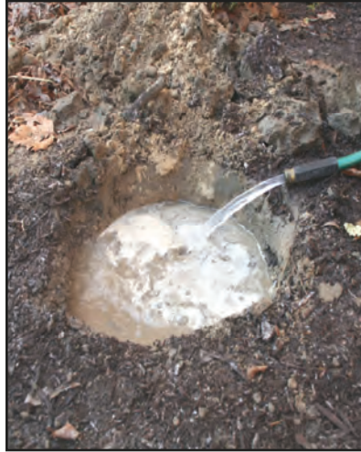
Figure 39. Fill the hole with water.
