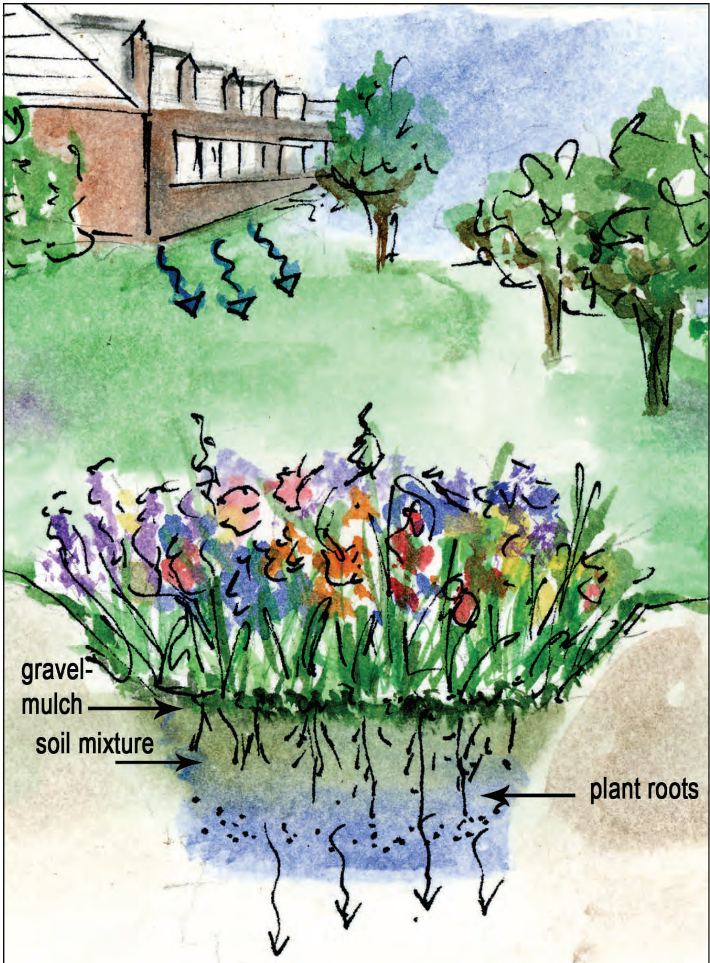
Figure 1. As runoff passes through the soil mixture, chemical and biological processes break down the pollutants. This helps protect the Atlantic Coastal and Chesapeake Bays from fertilizers, oils, and other pollutants carried by runoff.
