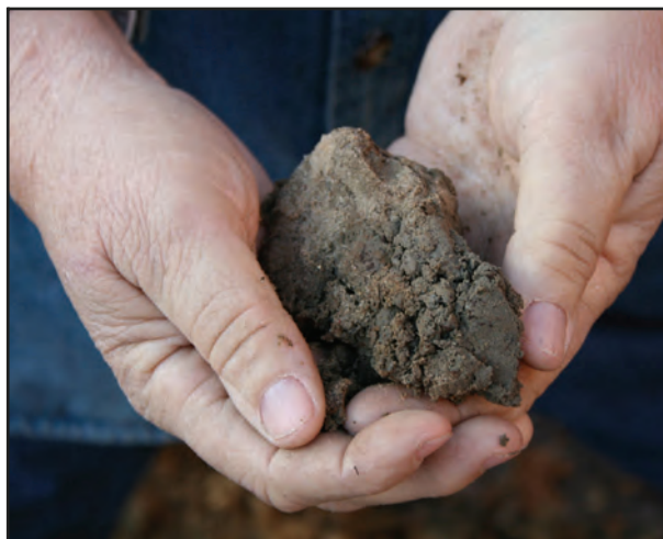
Figure 41. Dampen a handful of soil in your hands and knead the soil. Clay soil, when compacted, can prevent drainage. Sandy soil feels gritty and may be more difficult to knead, crumbling in the palm of your hands.
