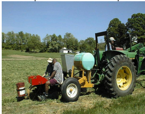
Figure 5. SST No-Till Transplanter setting tomatoes into a mown vetch-rye cover, Claggett Farm, Upper Marlboro.
