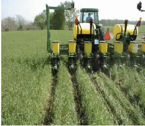
Figure 6. No-Till Planting into a rye cover with row cleaners aggressively set, USNAD.
