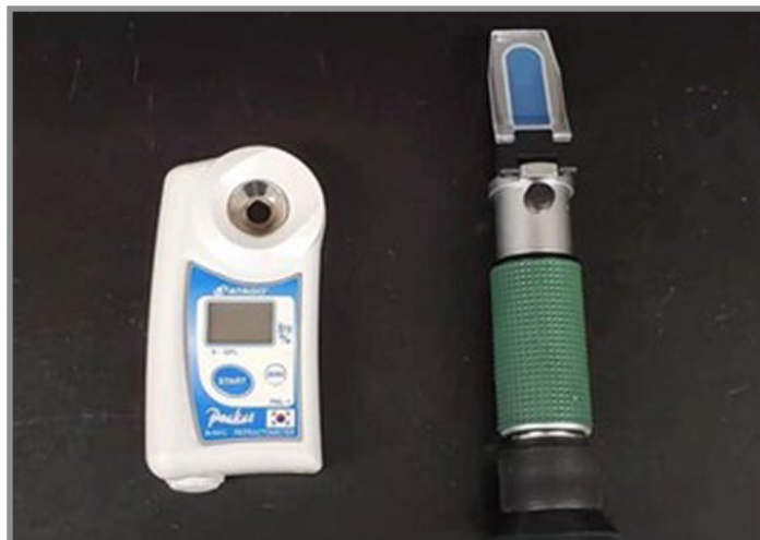
Figure 6. A hand-held manual refractometer (right) and digital refractometer (left) for measuring soluble solids contents of extracted peach juice sample. Source: Yixin Cai, University of Maryland
