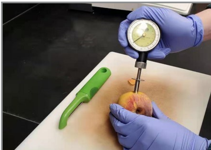
Figure 5. Using a hand-held penetrometer to measure the flesh firmness of peach. Source: Yixin Cai, University of Maryland
