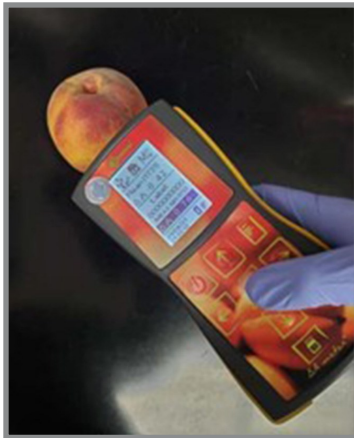
Figure 3. Using a DA meter to quantify the Index of Absorbance Difference ( I_{AD} ) in peaches which relates to the actual content of chlorophyll-a in the fruit skin. Source: Yixin Cai, University of Maryland
