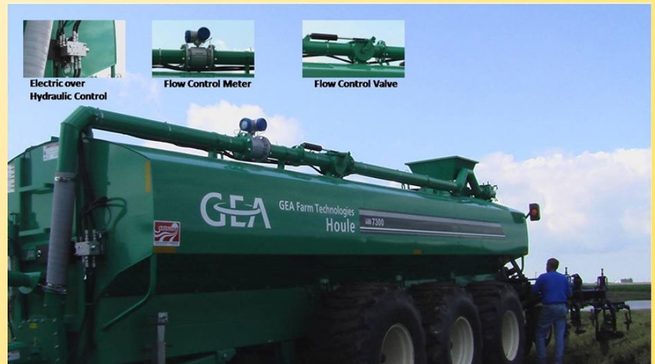
Figure 4 Commercial Applicator with Variable Rate Controls
