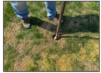
▲ Conducting a perk test to determine infiltration rates of site.
