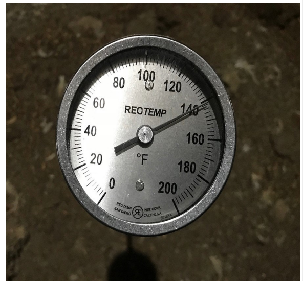
Figure 3. Use a compost thermometer to check litter temperature.
